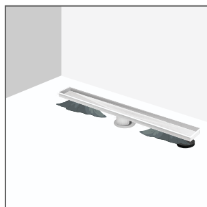
6. Pour the mortar mix into the bottom area of the drain base to provide support and guarantee the leveling.
