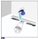
Perform a tightness test by pouring water into the drainage and check that the drain
