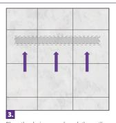
Place the drainage and mark the outline of the drain on the surface where you will perform the installation. The depth of the drainage with self-adjusting foot is from 2-5/8" to 3-3/8" (67 to 85 mm).
