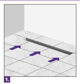
Determine the place where the linear drain/strainer will be installed. The position in the shower box can be at the back, front or center.
