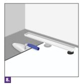
Spread the concrete mix up to the bottom edge of the drain base, generating a slope of at least 2% per linear meter, towards the place where it will be installed. If you wish, install a waterproofing membrane following the manufacturer's instructions.
