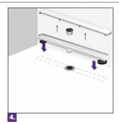
Connect the outlet tube of the drain base to the shower drain tube, sealing with impermeable silicone.
