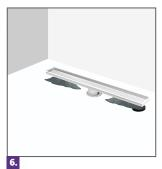
Pour the mortar mix into the bottom area of the drain base to provide support and guarantee the leveling
