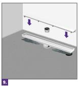
Place the hair strainer and the drain grate. For the 2-in-1 model, you may choose between the preselected smooth grate or invert it and place the ceramic tile in it.
