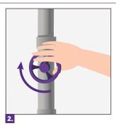
Close the outlet opening of the drain circuit before its mounting, to avoid the dirt produced during construction works from entering the duct.
