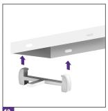
Remove the plastic fasteners using the hook and place them on the opposite side. Make sure they remain attached to the grate. For the ceramic tile version: apply a mortar layer inside the grate frame so that the ceramic tile is leveled with it.
