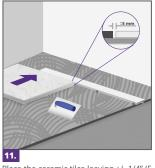
Place the ceramic tiles leaving +/- 1/4" (5 mm) of joint space with the edge of the drainage. To ensure the correct drain flow, the ceramic tiles must be placed 1 mm higher than the upper part of the drain. The installation can be performed with ceramic tiles of up to 5/8" high (16 mm). The edges of the porcelain tiles must be beveled. The sealing between the floor and the coating must be elastic and impermeable
