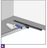
Spread the concrete mix up to the bottom edge of the drain base, generating a slope of at least 2% per linear meter towards the place where the drain will be installed. If you wish, install a waterproofing membrane following the manufacturer's instructions.
