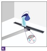
Perform a tightness test by pouring water into the drainage and check that the drain flows.
