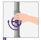
Close the outlet opening of the drain circuit before its mounting, to avoid the dirt produced during construction works from entering the duct
