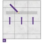
Place the drainage and mark the outline of the drain on the surface where you will perform the installation. The depth of the drainage is 3-3/8"(85 mm).
