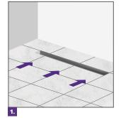
Determine the place where the linear drain/strainer will be installed. The position in the shower box can be at the back, front or center.
