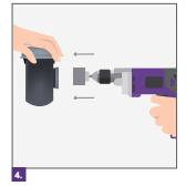
Make the hole in the corresponding outlet with a 1-3/8 or 1-7/16" (35 mm) hole saw.
