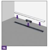
Place the inner siphon and the drain grate.
