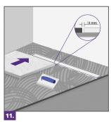
Install the ceramic tiles leaving +/- 1/4" (5 mm) of joint space with the edge of the drainage. To ensure the correct drain flow, the ceramic tiles must be placed 1 mm higher than the upper part of the drain. The installation can be performed with ceramic tiles of up to 3/8" high (9 mm). The sealing between the floor and the coating must be elastic and impermeable.
