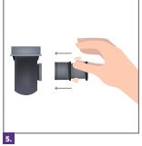
If necessary, connect the DM40/50 adapter to the outlet and insert it deeply to guarantee that the O-ring will retain any water seepage.
