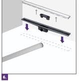
Connect the pipes of the drain network to the linear drain using glue on the connection.
