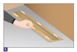
Stick the double-sided tape to the baseboard or skirting board backside with 2 cm/1" cuts every 40 cm/16" and no less than 20 cm/8" from the ends of the profile.
